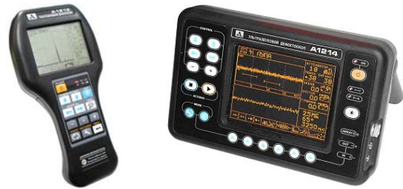
Fig. 19. Digital ultrasonic flaw detectors A1212 MASTER, A1214 EXPERT
