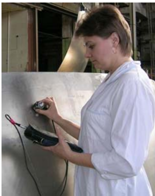
Fig.16. Process of thickness measurement
