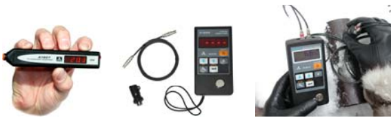
Fig. 15. Digital ultrasonic thickness gauges A1207, A1208, A1209
